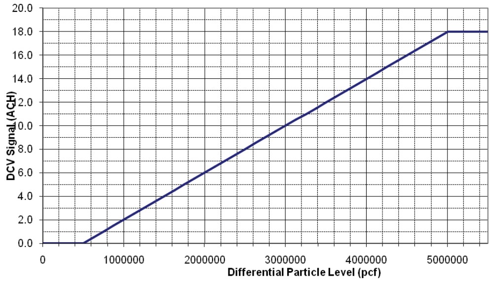
DCV Signal vs. Differential Particle Level y = (4.0 \times 10^{-6})x - 2
